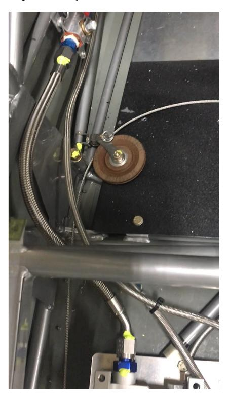
3. Hose #3 – "ASF 21-901 R(X) H3" – This hose has a 45 degree fitting on one end and a Straight on the other. This hose goes between the fuel valve and the firewall. The 45 degree fitting is utilized at the firewall and angles the hose toward the left side of the cabin.
